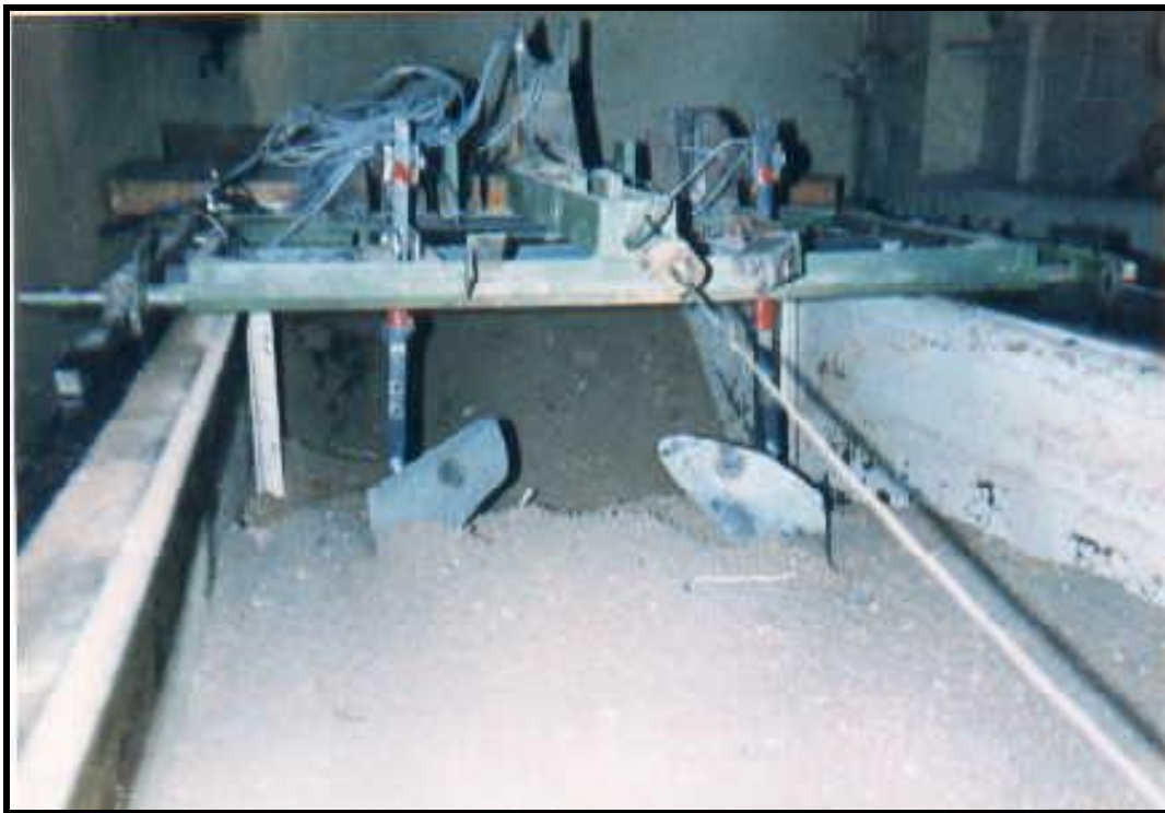
Figure 5. Small-scale ploughs models assembled on channel of traction.
